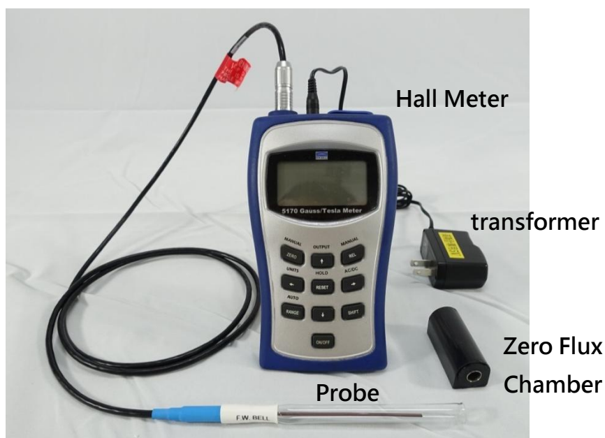
Figure 1. Photo of a Hall Probe Meter
